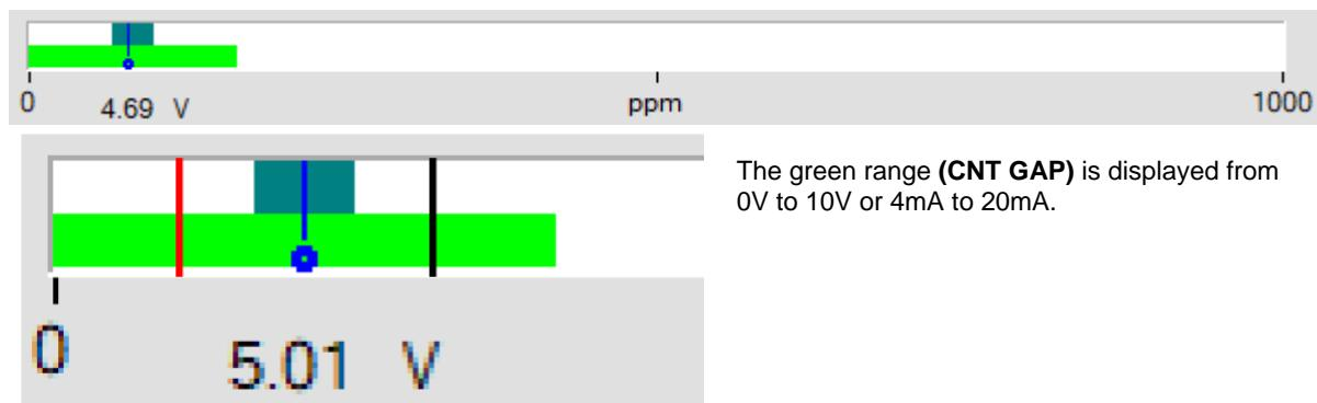
If the cursor (**punch stroke CNT STROKE**) is on the position of the blue line, 5V or 12mA is output.
