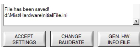
A click on the **GEN. HW INFO FILE** generates a file in which all the important sensor data are stored in encrypted form. This file can be sent to the manufacturer for diagnostic purposes.
